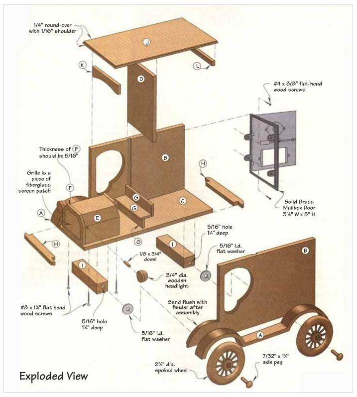
steering-wheel column and headlights (see *Hood drawing*). Lay out a centered dowel hole on each headlight. Clamp each one into a handscrew clamp laid flat on the drill press table, set the depth stop, and drill a 1/8" hole 3/8" deep. Glue the steering wheel to the column, then glue the column into its hole. Cut two 3/4" lengths of 1/8" dowel, and glue one into each headlight. Glue the dowels into the hood, and level the headlights.
